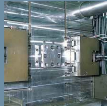
C-plate clamp unit Eliminates the need for push rod installation for die changing.
