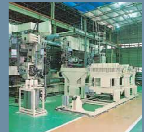
Die loading unit Use of guide rollers for lateral transfer of die into machine eliminates the use of a crane for greatly reduced setup time.
