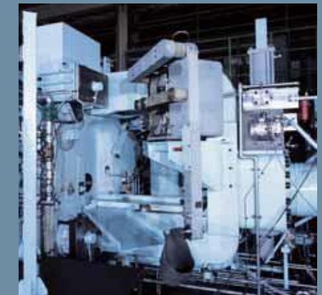
Automatic Ladle Device New ladle device for large-sized machines, pursuing an improved ladling accuracy and fast cycles.
