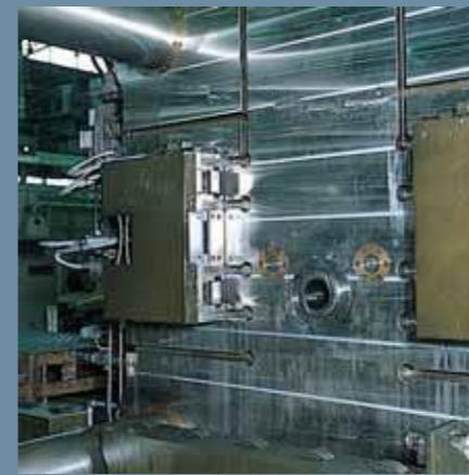
Die clamp Uses hydraulic pressure clamping and a self-locking mechanism.
